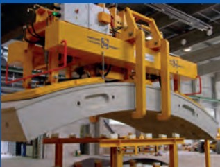
Emscher sewer tunnel – pipe factory, Gelsenkirchen, Germany, Lifting beam for concrete pipe segments
