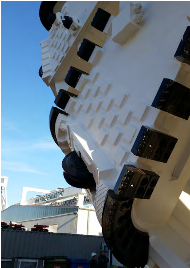
4 Verschleißschutz in Form von Aufpanzerungen am Schneidrad Wear protection in the form of reinforcements on the cutting wheel
