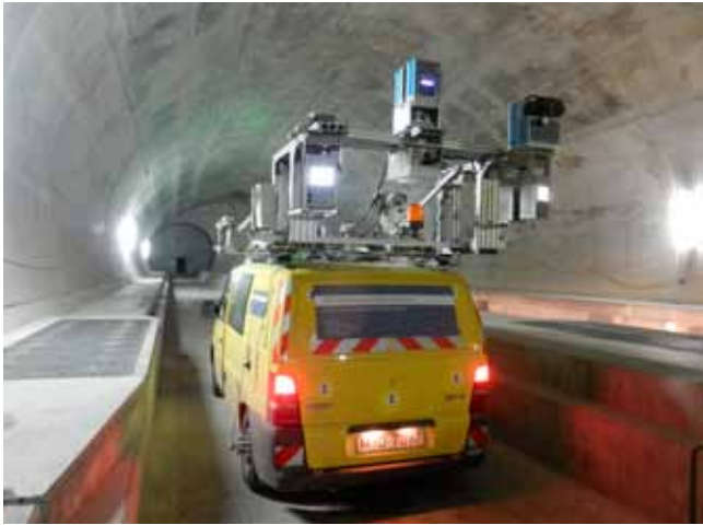
Mobiles terrestrisches Laserscanning-System Mobile terrestrial laser scanning system
