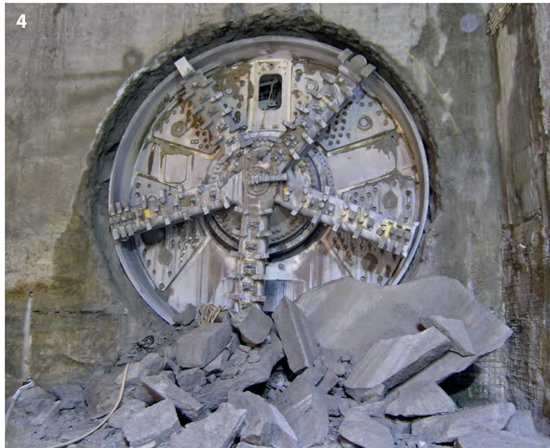
U-Bahn in München: Offenes Speicherschneidrad der TVM Munich Metro: open spoked cutting wheel for the TBM
