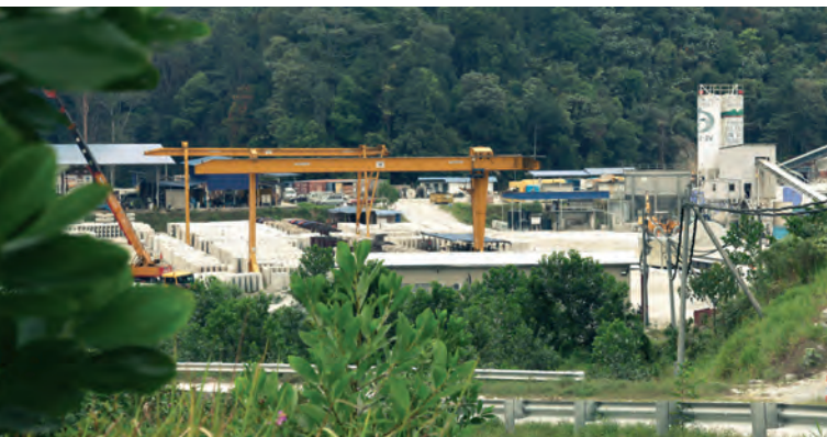
Remote adit sites are located in the mountains surrounding Kuala Lumpur, Malaysia, requiring supplies such as invert segments to be cast onsite
