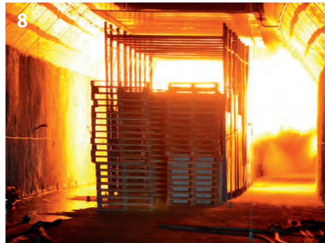
Full-scale fire tests (over 200 MW HRR before triggering FFFS) [8]
