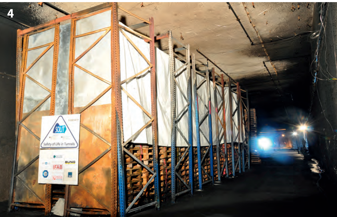
Tarpaulin – covered HGV (truck) fire mock-up [13]
