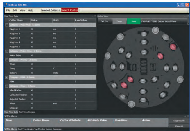
In this hypothetical illustration, an operator sees flagged cutters that are above a threshold limit indicating the presence of a fault zone
