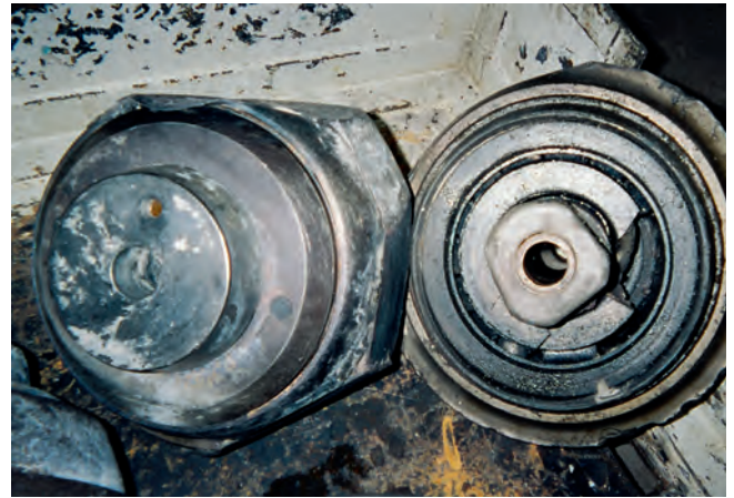
Cutter wipe outs caused when cutters become blocked can be monitored and prevented using real-time rotational data
