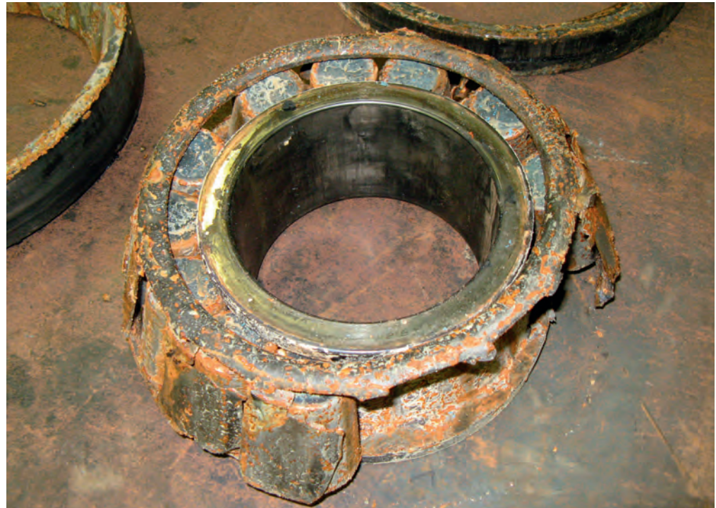
The cutter monitoring system detects anomalies such as a non-turning cutter, preventing problems such as failed cutter bearings (pictured)
